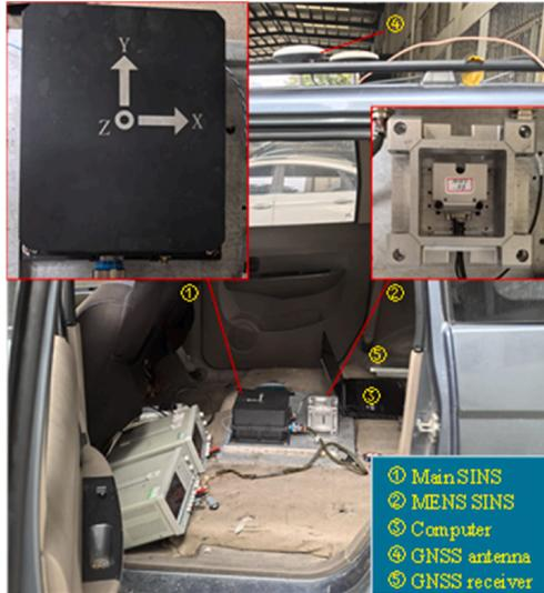
Fig. 10. Equipment used in the road test.
